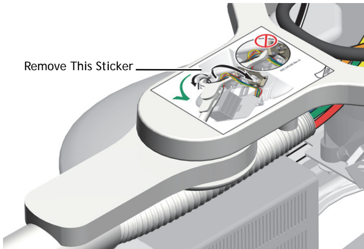
Figure 66. Remove the Routing Sticker
