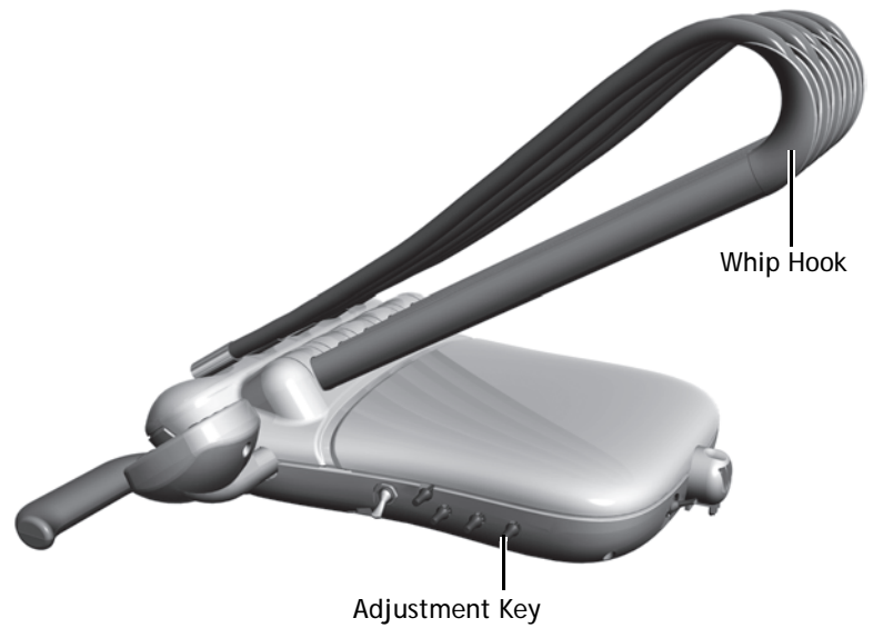
Figure 48. Insert Whip Hooks and Adjustment Keys
