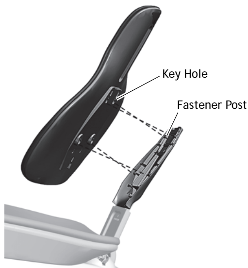
Figure 95. Install the Back Upholstery
