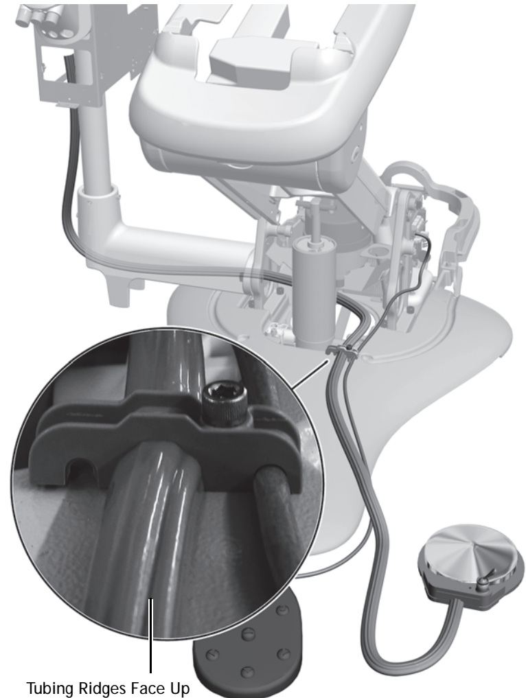
Figure 90. Secure the Foot Control Tubing
