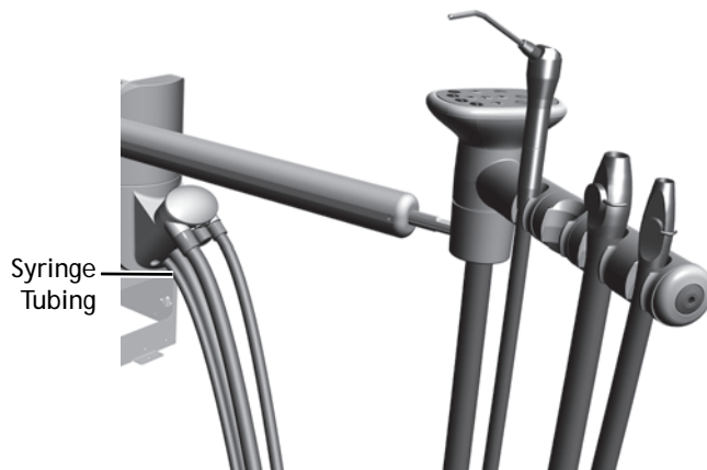
Figure 33. Route the Syringe Tubing
