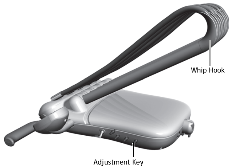
Figure 41. Insert Whip Hooks and Adjustment Keys
