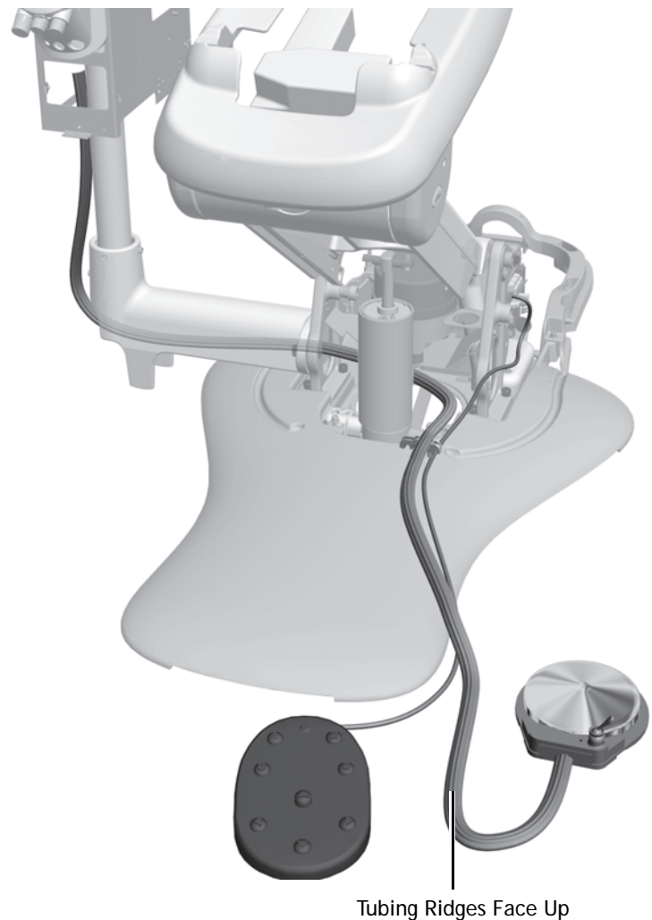
Figure 49. Route the Foot Control Tubing
