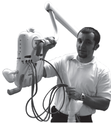
Figure 46. Carry the Delivery System
