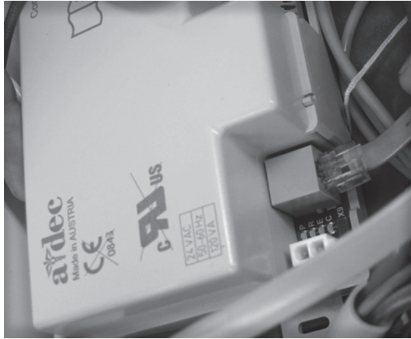
Figure 26. Plug in the Data Line
