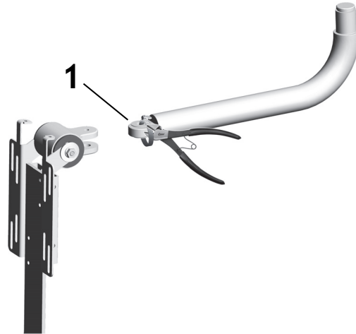
Figure 2. Attach the Hub Assembly to the Trolley Arm
